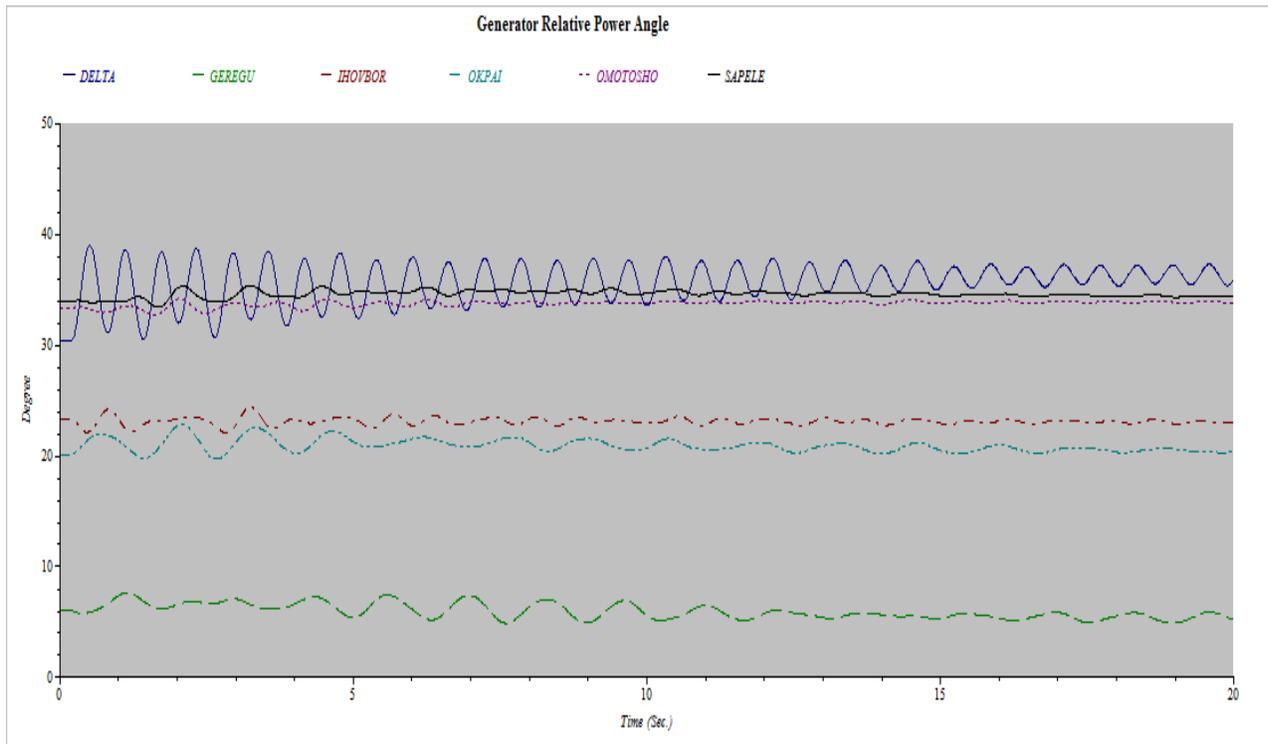
**Figure 4.2: Plot of Generator Relative Power Angle with Time**
