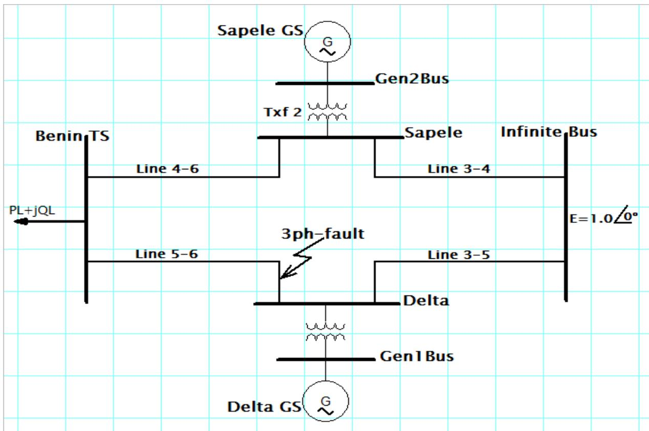
Figure 3.5:Network Model of Nigeria 330kV Grid
