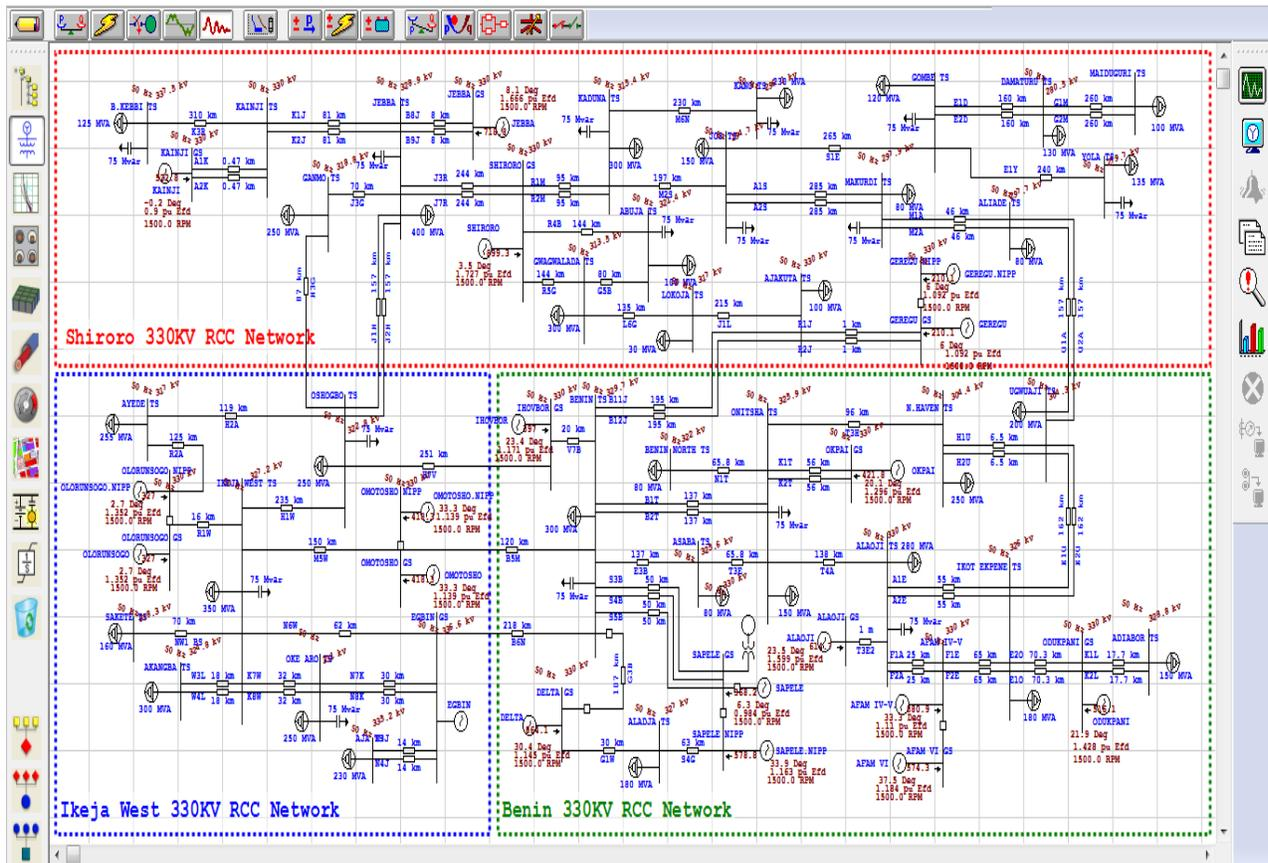
**Figure 4.1: Model of the Existing Nigeria 330kV Network after Simulation**
