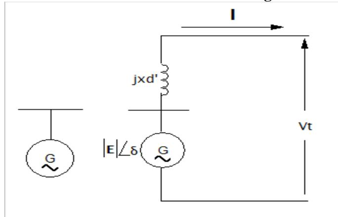
Figure 3.2: Synchronous Machine Model
