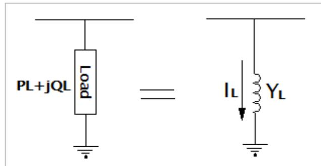
Figure 3.3: Static Load Model
